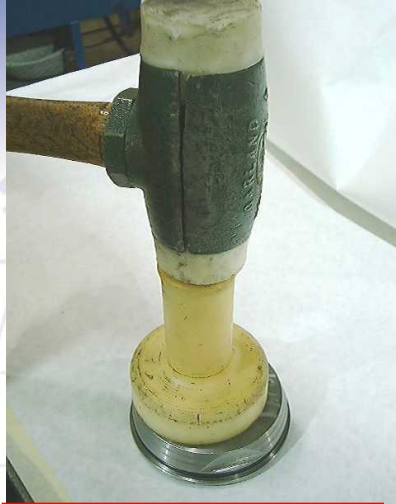
INSTALL SEALS WITH A SEAL DRIVER TO PREVENT DAMAGE
